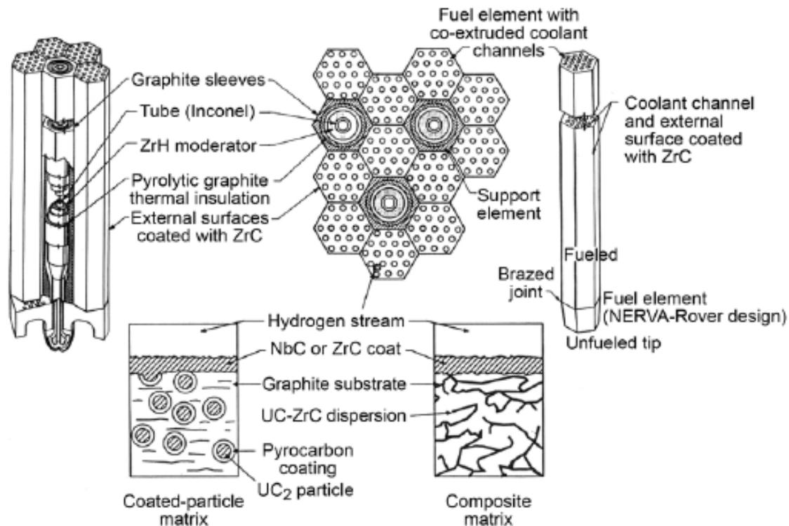
Figure 1-4. Coated particle and composite SNRE fuel element and tie tube arrangement.
