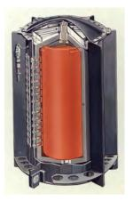
**Figure 9.** Cutaway of the MHW-RTG which was used on LES 8/9 and Voyager 1/2. The overall diameter was 39.73 cm and the length was 58.31 cm. The average flight mass for Voyager 1/2 was 37.69 kg. (ERDA/GE)
