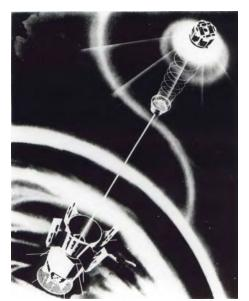
**Figure 5.** Artist's conception of the Transit 5BN-1 navigational satellite in orbit. The SNAP-9A RTG is mounted at the lower left in this drawing. Transit 5BN-1 was the first spacecraft to be totally powered by a nuclear power source. Transit 5BN-1 was an octagonal prism 45.7-cm across by 30.5-cm high. (JHU/APL)
