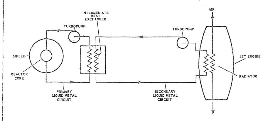
IN THE INDIRECT CYCLE, THE HEAT GENERATED IN THE REACTOR IS ABSORBED BY A LIQUID-METAL COOLANT FLOWING THROUGH THE REACTOR CORE. THE LIQUID-METAL COOLANT THEN FLOWS THROUGH AN INTERMEDIATE HEAT EXCHANGER WHERE THE HEAT IS TRANSFERRED TO A SECONDARY LOOP. THE HOT LIQUID METAL IS THEN PUMPED TO THE JET ENGINE. THE JET ENGINE CONTAINS RADIATORS, WHERE THE HEAT IS GIVEN UP BY THE LIQUID METAL AND IMPARTED TO THE AIRSTREAM FLOWING THROUGH THE ENGINE.
