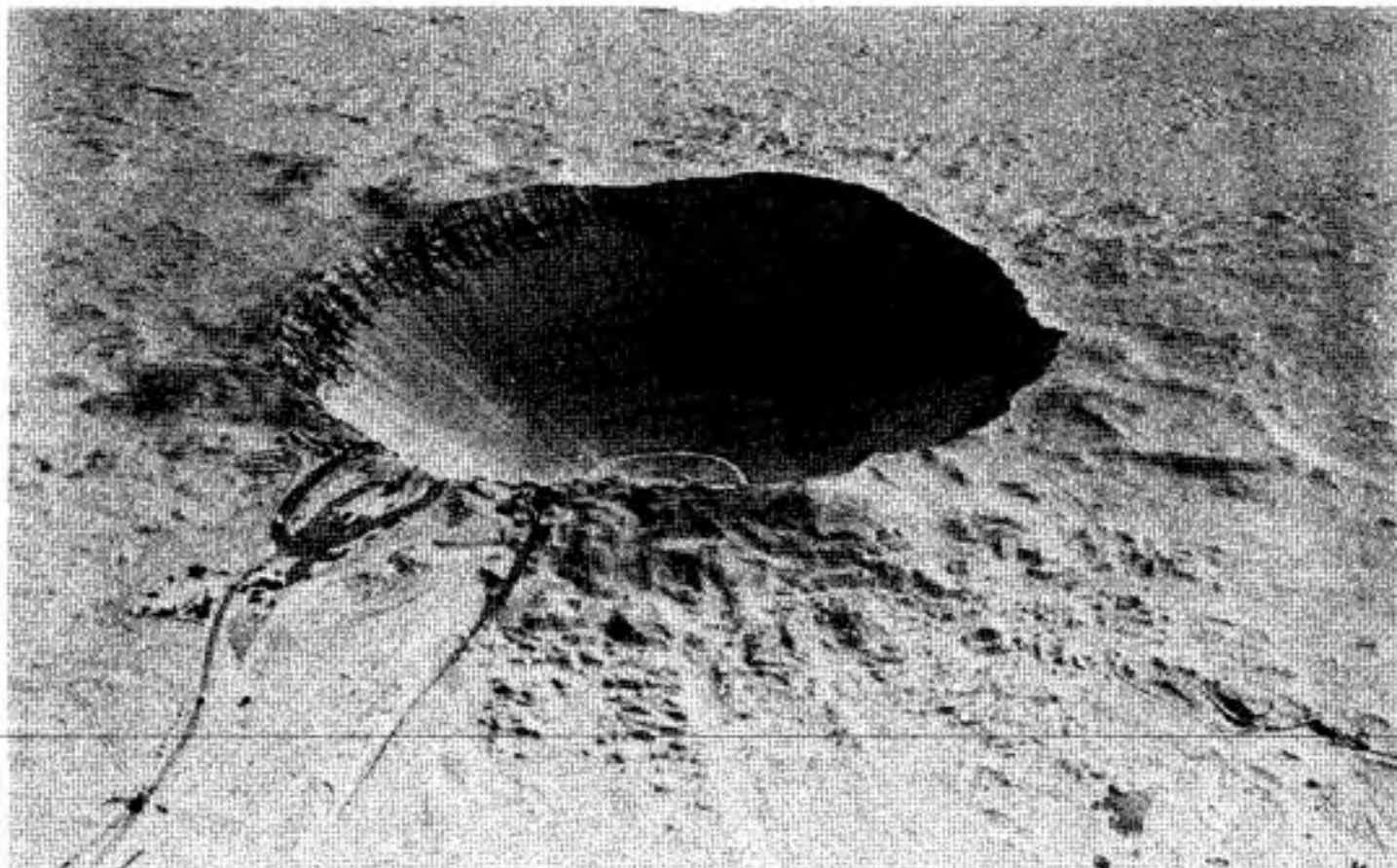
Figure 2 20 Sedan Crater, Yucca Flat, Nevada Test Site, (view is to the north-northeast) Crater diameter is 370 m, depth 98 m, and volume 5.0 \times 10^6 \text{ m}^3 . Crater formed in 1962 by a 100 \pm 15 kiloton
