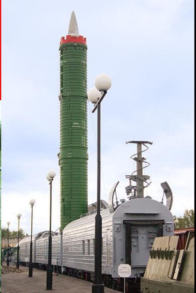
RT-23 / SS-24 Scalpel ICBMs had 10 MIRV warheads with design yields of 550 KT. The system was extremely heavy, so heavy that it caused extensive rail damage when deployed. This problem likely was one reason the Russians agreed to retire the RT-23 under the SALT agreement.
