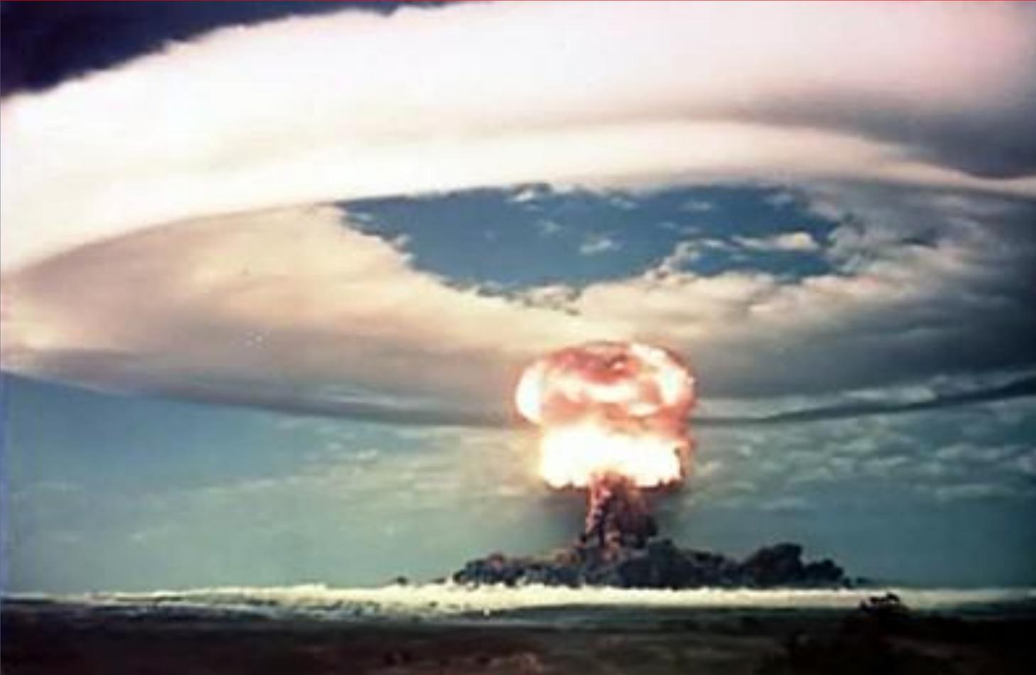
RDS-4 (JOE-5) was a fission device using plutonium in a "levitated" core design. The test was an air drop on August 23, 1953, yielding 28 KT.
