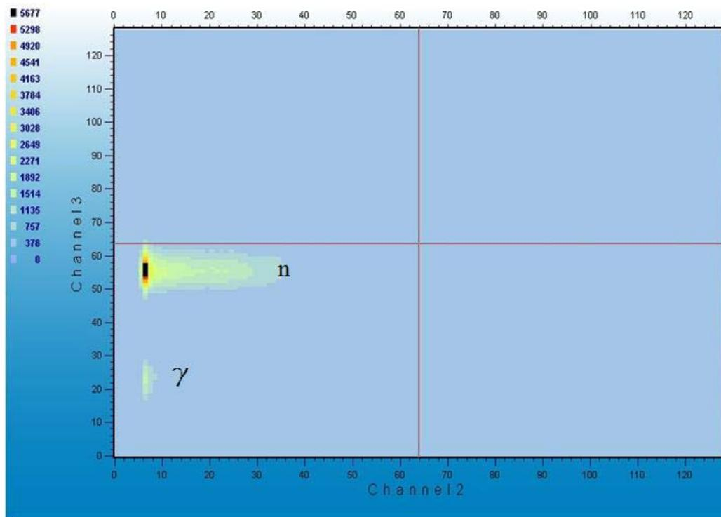
Fig.(7). Neutron gamma discriminated spectra from 0.5 mm target.
