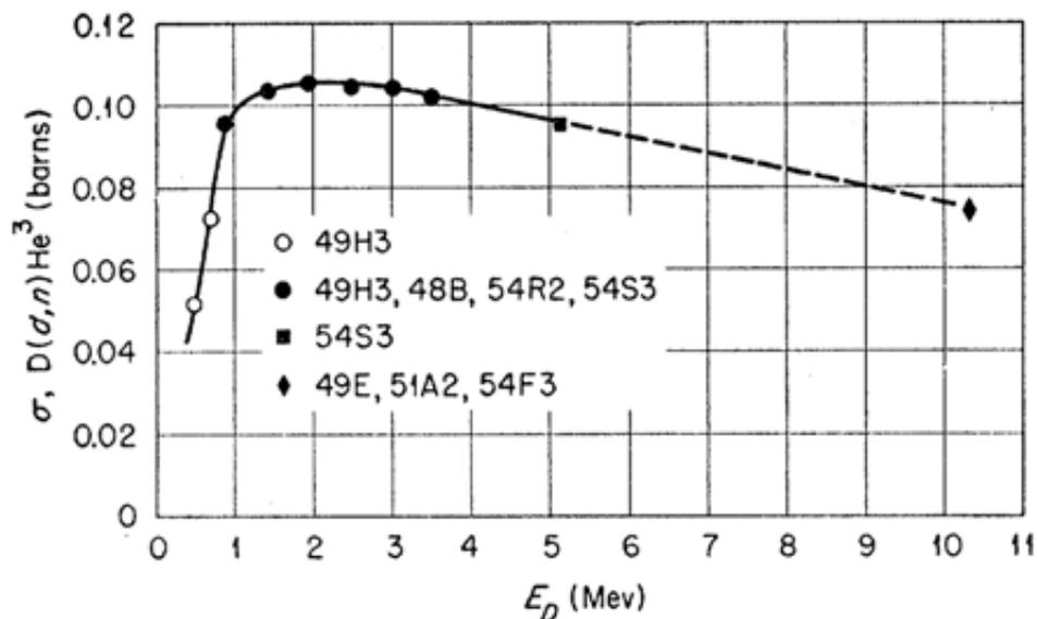
Fig (9). Cross section of D-D reaction according to incident deuterium energy [6].
