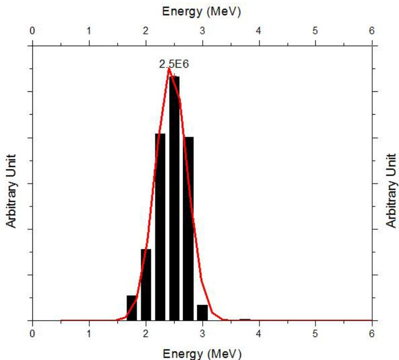
Fig.(8) .Final neutron energy spectra from bombardment of 0.5 mm target by d-D reaction.
