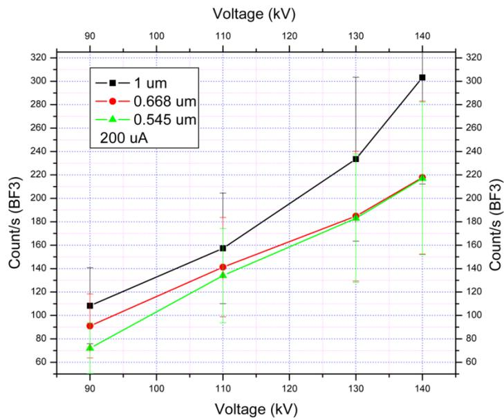
Fig(2). Count rate of BF<sub>3</sub> v.s voltage (200  $\mu$ A)
