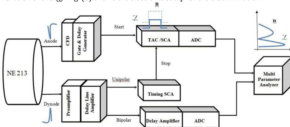
Fig. (6) Set up of the neutron-gamma discrimination.
