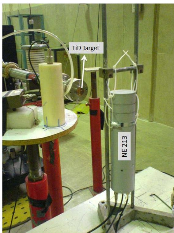
Fig. (5). the situation of the target and the scintillator. The scintillator has been set to the zero degree respect to the incident D beam.
