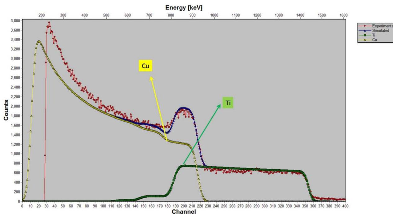
Fig(1). RBS Spectra of 1<sup>st</sup> target for measuring the thickness of titanium layer.
