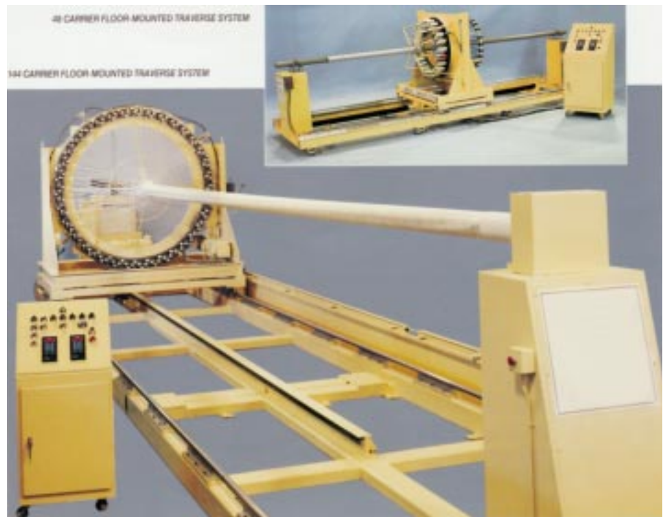
Figure 6-7: A 144 carrier floor-mounted traverse braiding machine.
