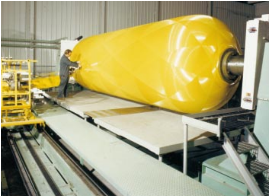
Figure 6-2: A large multi spindle filament winding machine.
