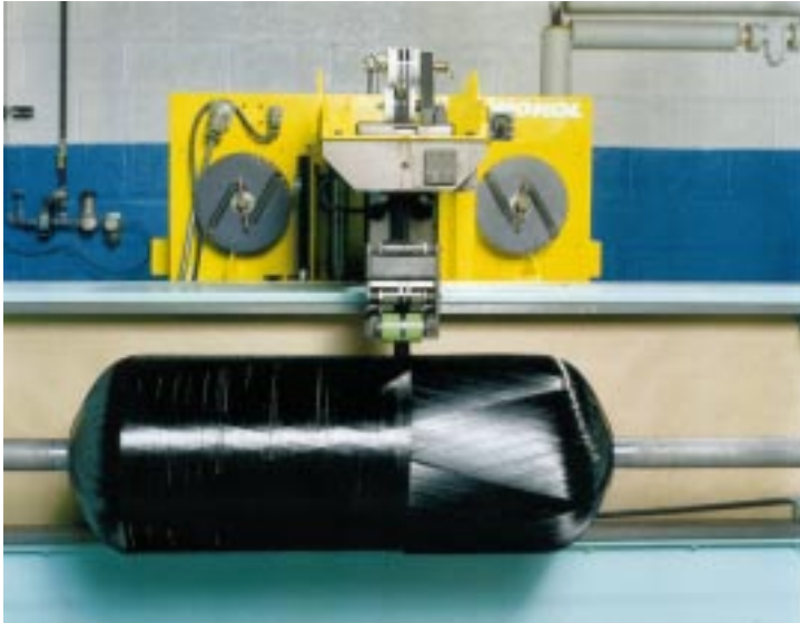
Figure 6-1: Tabletop filament winding machine.
