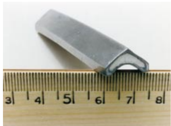
Figure 3-28: Short section of flexible linear-shaped charge (on a centimeter scale) designed to cut through a missile stage.
