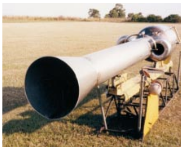
Figure 3-10: A modern pulsejet engine with a rearward-facing intake.
