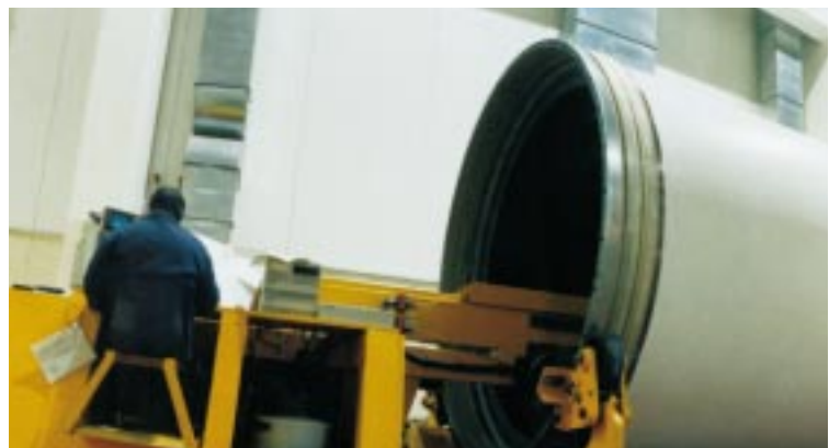
Figure 3-19: A rocket case under inspection after application of the thermal insulation.
