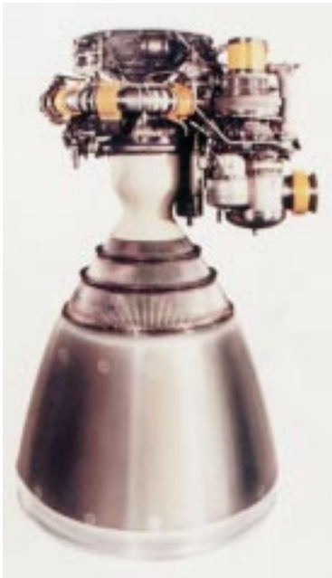
Figure 3-21: A liquid engine with a metal, radiatively cooled lower nozzle skirt.
