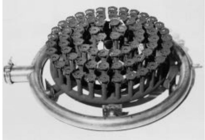
Figure 3-14: A fuel manifold and centrifugal fuel injector assembly for a ramjet engine.
