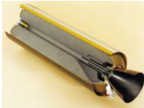
Figure 3-22: A cut-away view of a solid motor that shows how the nozzle fits into the aft end of the motor.
