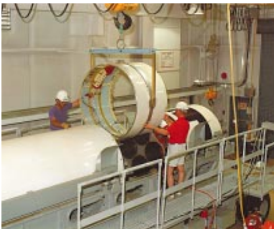
Figure 3-30: An interstage being positioned for attachment.
