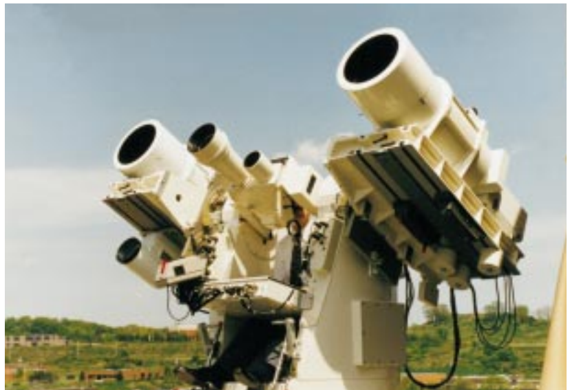
Figure 12-29: An optical missile tracking system.
