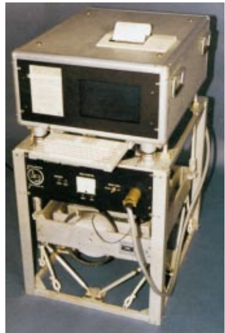
Figure 12-13: Complete non-MTCR-controlled air-sea gravity meter system with mini-console.
