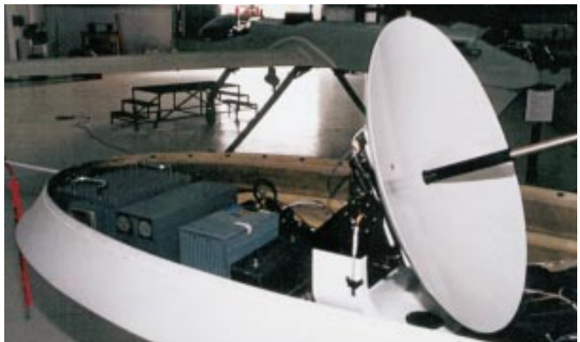
Figure 12-21: A SATCOM antenna installed in an unmanned air vehicle.
