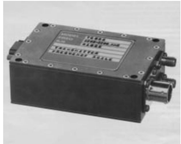
Figure 12-16: Telemetry transmitters for installation in flight vehicles.
