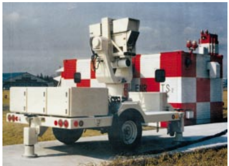
Figure 12-31: A mobile laser missile tracking system.
