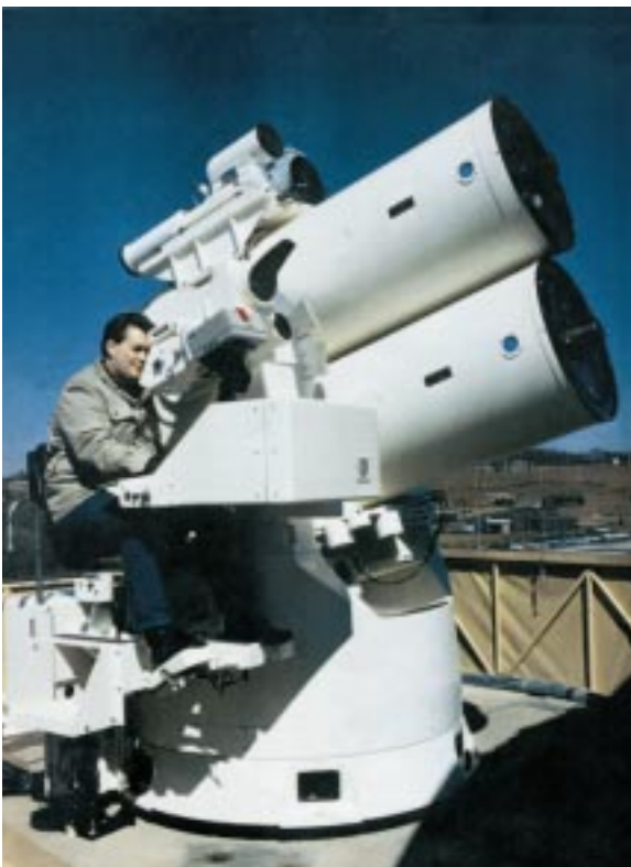
Figure 12-30: An optical missile tracking system.
