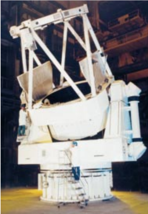
Figure 12-28: An optical missile tracking telescope.
