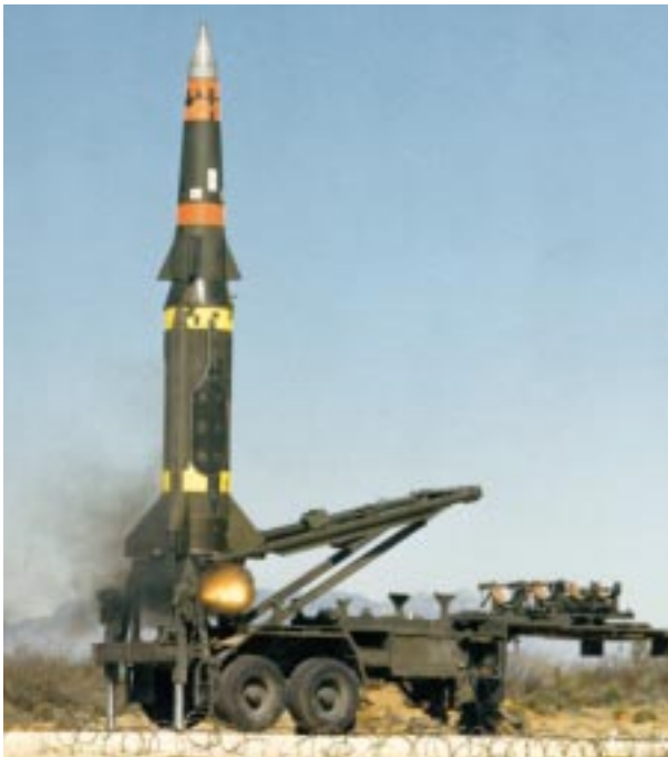
Figure 12-4: An erector launcher detached from its prime mover.
