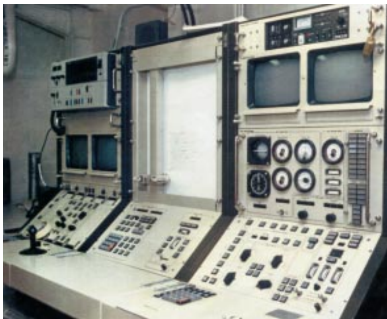
Figure 12-26: An integrated unmanned air vehicle control station.
