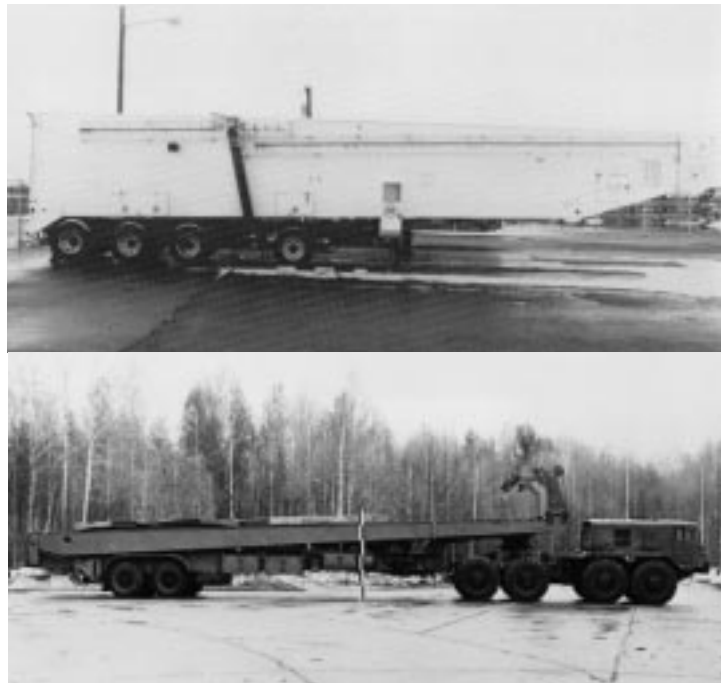
Figure 12-5: Two different approaches to silo-based missile transporter and installation vehicles.
