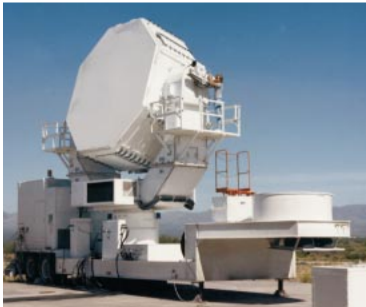
Figure 12-27: A mobile phased array missile tracking radar.
