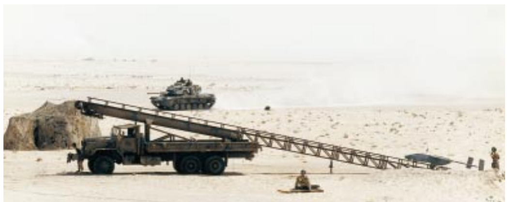
Figure 12-9: A pneumatic unmanned air vehicle launcher.
